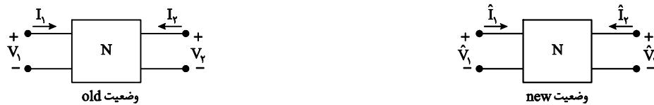
$$V_{1,old} \hat{I}_{1,new} + V_{2,old} \hat{I}_{2,new} = \hat{V}_{1,new} I_{1,old} + \hat{V}_{2,new} I_{2,old}$$
